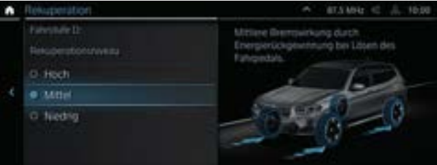
■ The recuperation system converts the kinetic energy generated during deceleration into electricity and feeds this into the drive's high-voltage battery.
