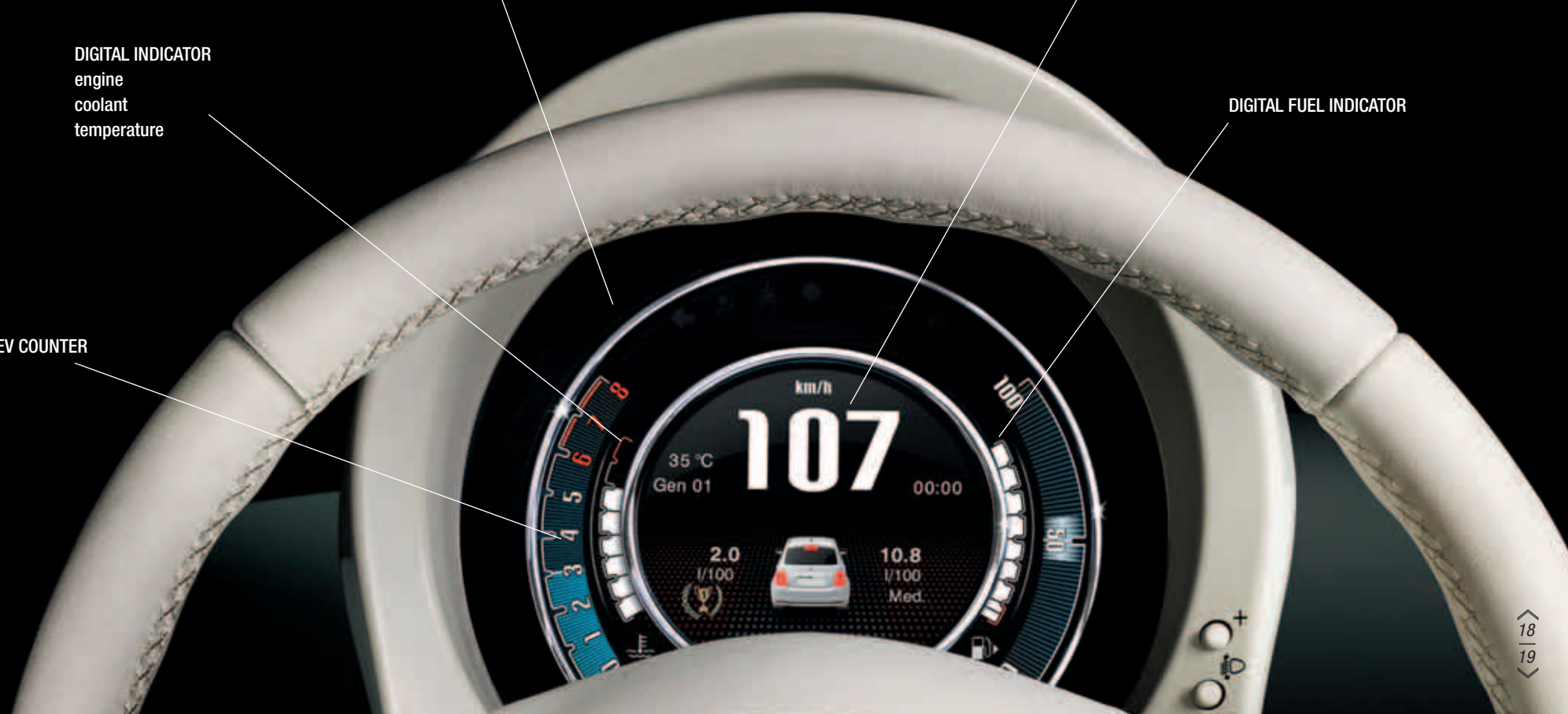
HMI (Human Machine Interface) in the integrated display with the rest of the on-board electronics
